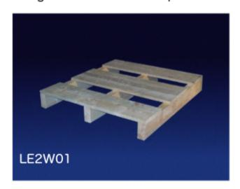
A pallet with only a top deck. Suitable for items that can withstand the concentrated loads imposed by the bearers during stacking, e.g, wooden boxes and drums. Also used where little stacking is required and for storing unit loads in pallet racking when the bearers are supported by the rack framework.
